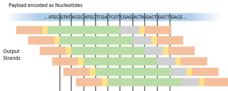
Fig. 6. The Goldman encoding uses fourfold redundancy of each segment.
